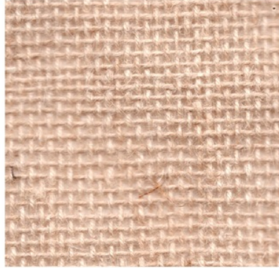
Figure 1. Ramie plain weave fabric model with 12S/3 yarn type
