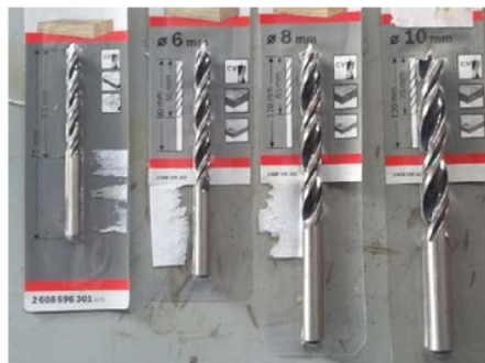
Figure 2. “Brad & spur” drill diameter 4, 6, 8 and 10 mm
